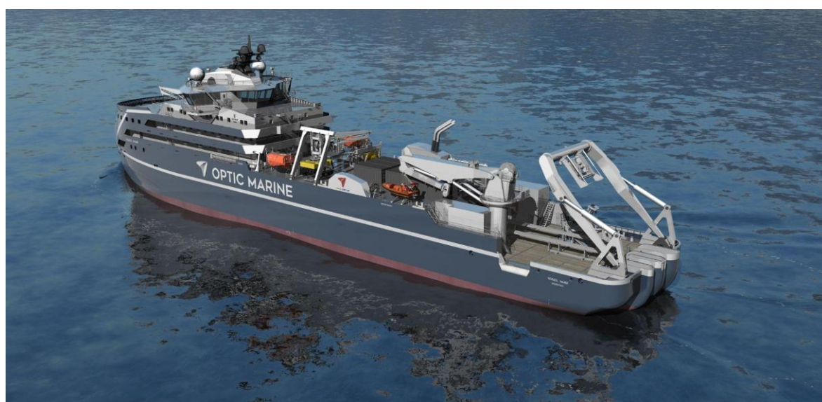
Figure 1 An illustration of a cable ship capable of installation and repair. (Image: Ulstein 1 )
