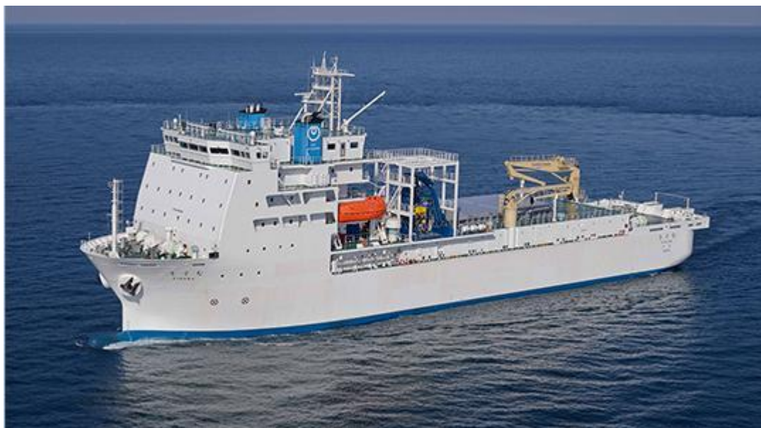
Figure 10 NTT WEM's Kizuna was designed as a multi-purpose vessel used for cable laying and maintenance as well as disaster relief. (Source: NTT WEM 67 )
