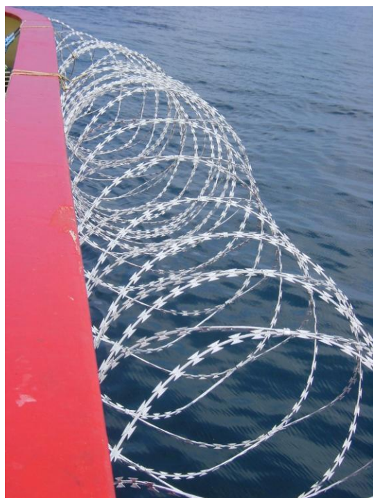
Figure 8 Razor wire installed on a cable ship. An example of on-board fortifications. (Source: Image courtesy of Steven Onley)
